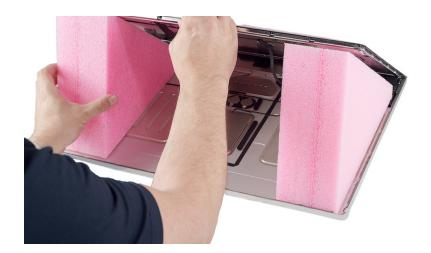
Note: Use the VESA support slot wedge and two triangle support wedges for models configured with a VESA mount adapter.
