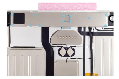
4. Tilt up the logic board cover. Then pull it toward you to remove it from the housing.
