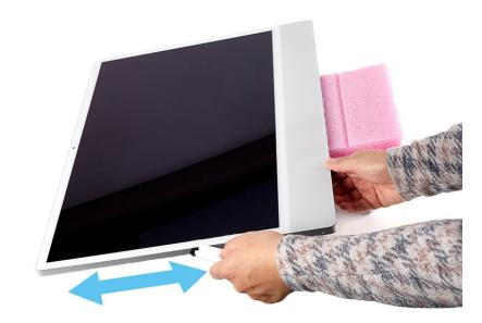
4. Run the adhesive cutter between the display and housing on the bottom edge of the computer.
