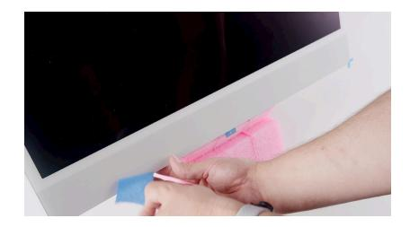
23. Separate the display from the housing just enough to remove the release liners from the four display adhesive strips on the bottom half of the computer. Start near the middle and peel the release liners toward the bottom corners of the computer in the order shown.
