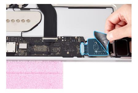
2. Use the T3 screwdriver to remove the two T3 screws (923-05555) from the USB-C board.
