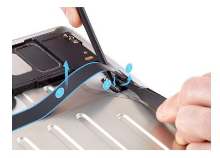
3. Use the T3 screwdriver to remove the upper three T3 screws (923-05574) and the lower T3 screw (923-05668) from the Wi-Fi and Bluetooth antenna.
