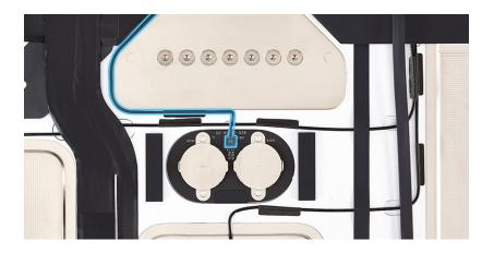
3. Use ESD-safe tweezers to grasp the battery adhesive tab and gently peel it from the battery board.
