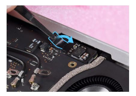
5. Use the black stick to flip up the locking lever on the end of the fan flex cable connectors.
