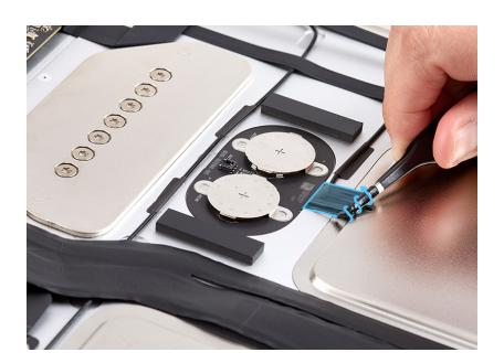
5. Pull the tweezers down. As the battery adhesive strip stretches, continue to slowly pull and twist the tweezers until you have removed the entire strip.
