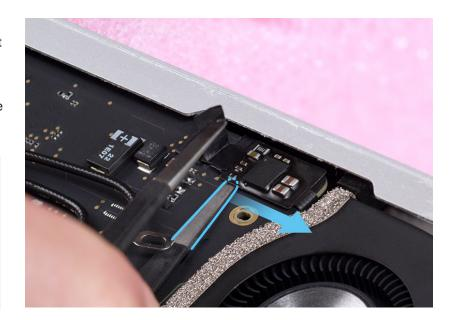
7. Position the black stick under the fan flex cable. Then pull the fan flex cable out of the connector.
