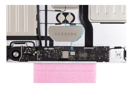
8. Use the T3 screwdriver to remove two long T3 screws (923-05173) from the overlapping antenna grounding clips.
