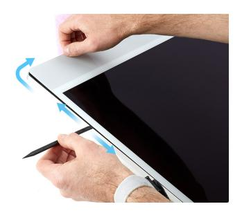
7. Rotate the computer so the top edge of the display is closest to you. If fully released, the display will extend slightly over the top edge of the housing.
