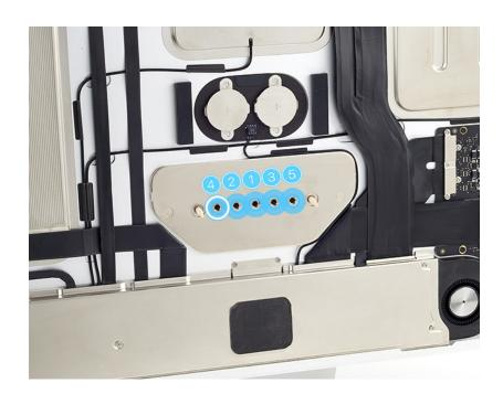
8. Remove the alignment pins by rotating them counterclockwise and pulling them out of the housing.
