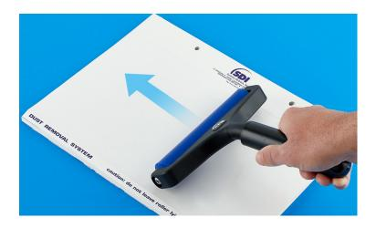
28. Roll the silicone roller back and forth along all four edges of the display to adhere the display adhesive strips.
