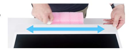
5. Run the adhesive cutter back and forth between the display and housing around all four edges of the computer until the wheel moves with minimal resistance.
