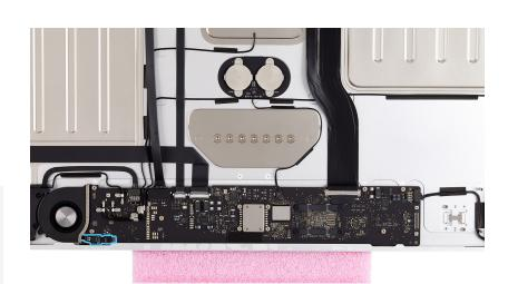
18. Slide the camera and eDP flex cable into the connector (1). Then flip down the locking bar (2).
