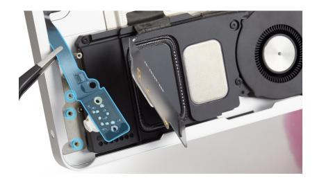
2. Use the T3 screwdriver to partially reinstall the upper T3 screw (923-05670) and the lower T3 screw (923-05669) into the audio board.
