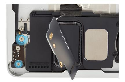
7. Use the 3.5 mm hex nut driver to remove the 3.5 mm hex screw (923-05671) from the audio board.
