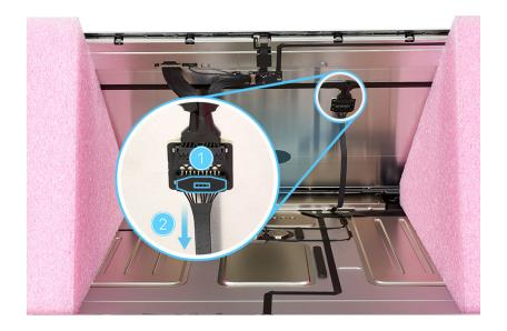
12. Flip up the locking levers of the camera and embedded DisplayPort (eDP) flex cable connectors (1). Slide both ends of the eDP flex cable out of their connectors (2).
