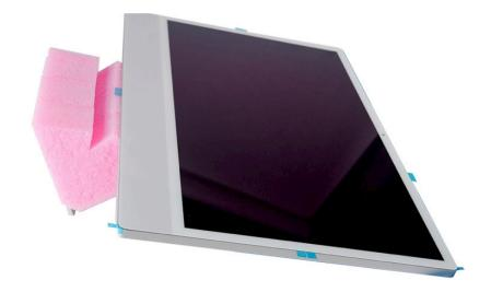
16. Apply two strips of painters tape to the bottom of the computer to temporarily secure the display to the housing.
