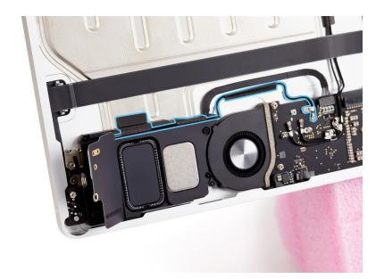
5. Press the antenna cable tape back onto the speaker and housing.
