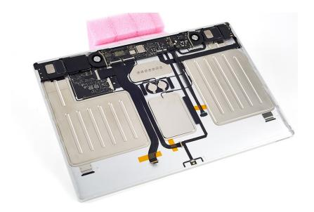
2. Gently peel up the polyester film tape attached to the housing in the area shown. Don't remove the tape from the battery board cable. Remove the cable from the housing.
