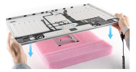
4. Slide the housing onto the alignment pins. Ensure the alignment pins enter the outer screw holes of the housing.
