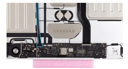
13. Slide the end of the microphone flex cable into the connector.
