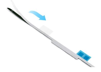
2. Lay the housing flat as shown. Peel off a short section of the paper release liner from one display adhesive strip.
