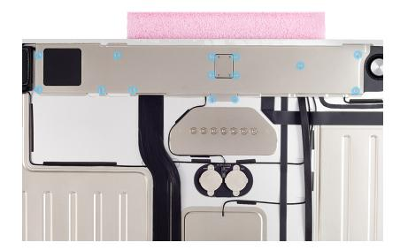
4. Adhere the tape onto the middle of the logic board cover.
