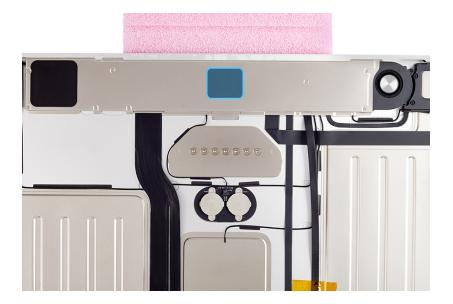
3. Use the T3 screwdriver to remove the 14 T3 screws (923-05557) from the logic board cover.
