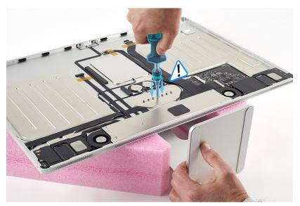
4. Remove the flange and stand from under the housing.
