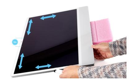
6. Insert the flat end of the black stick halfway to its notch between the display and housing. Slide the black stick up and down to cut any remaining adhesive.
