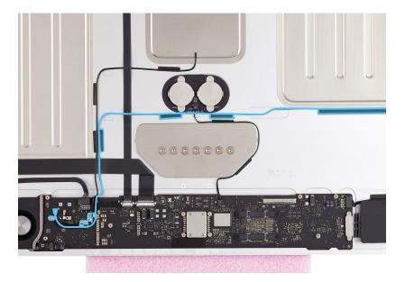
5. Carefully lift the cable out of the channel in the speaker.
