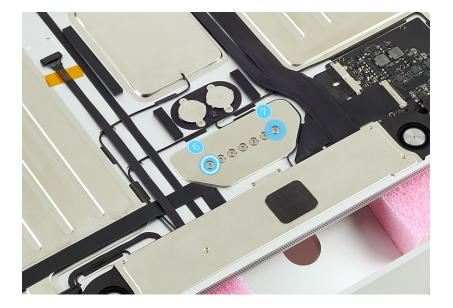
11. Keep the Torx Plus 10IP bit in the 1.2–3 Nm adjustable torque driver. Ensure that the torque value is still set to 1.4 Nm.
