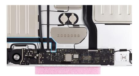
15. Press the end of the battery board cable onto the connector.
