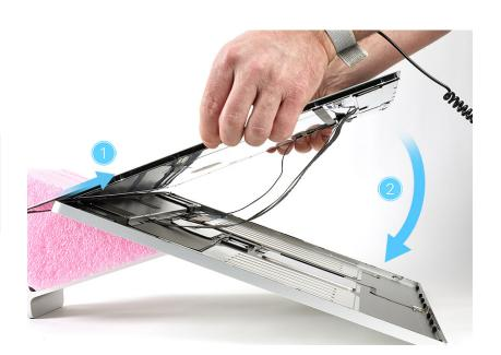
15. Position the display flat on the housing. The top edge of the display should hang just over the top edge of the housing.
