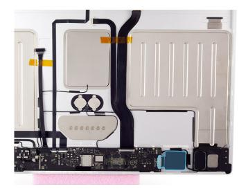
1. Peel the polyester film tape from the USB-C board. Save it for reassembly.
