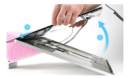
10. Insert the two triangle support wedges into the housing as shown.
