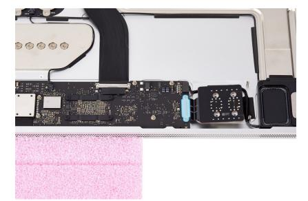
5. Use the black stick to lift the end of the USB-C board flex cable off the connector. Then remove the USB-C board from the housing.
