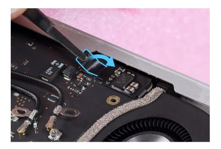
22. Use the black stick to flip up the locking lever on the fan flex cable connector.
