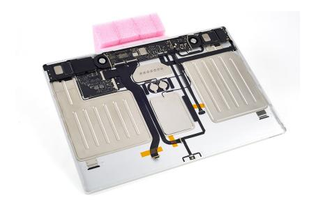
21. Use ESD-safe tweezers to peel off the polyester film tape on the fan flex cable.
