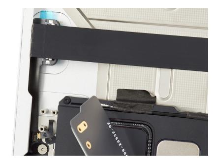
8. Slide the end of the audio board flex cable into the ZIF connector.
