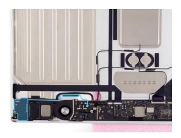
1. Use the T3 screwdriver to remove the upper three T3 screws (923-05574) and the lower T3 screw (923-05668) from the Wi-Fi and Bluetooth antenna.
