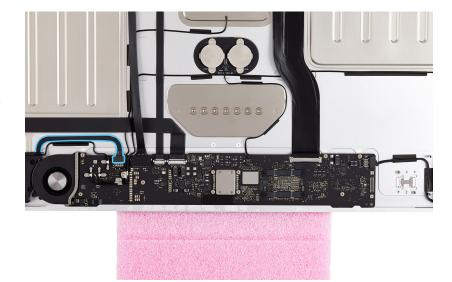
3. Peel off the polyester film tape from the display backlight flex cable connector. Save the polyester film tape for reassembly.
