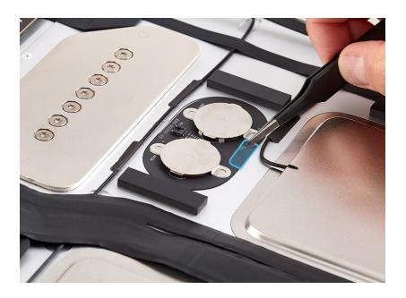
4. Use ESD-safe tweezers to grasp the battery adhesive tab. Keep the tweezers close and parallel to the housing. Then slowly twist the tweezers to wrap the adhesive around them.
