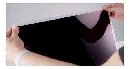
21. Apply two strips of painters tape to the top of the computer to temporarily secure the display to the housing.
