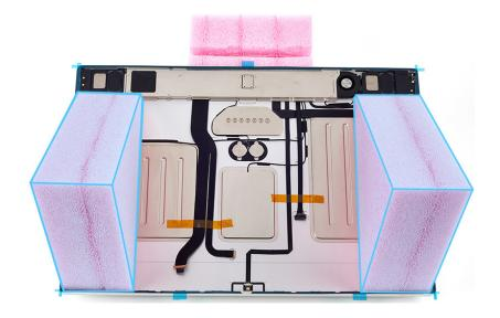
9. Insert the bottom edge of the display into the slot in the stand support wedge. Rest the display on the triangle support wedges.
