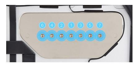
7. Use the adjustable torque driver and Torx Plus 10IP bit to fully reinstall the seven 10IP screws in the order shown.
