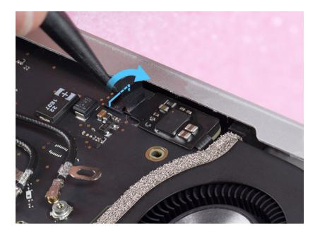
6. Separate the prongs of the ESD-safe tweezers and insert one prong under the fan flex cable. Carefully slide the ESD-safe tweezers toward the fan to loosen the adhesive between the fan flex cable and the logic board.
