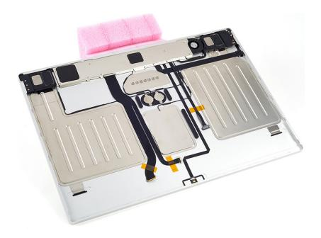
2. Peel the tape off the middle of the logic board cover. Save the tape for reassembly.
