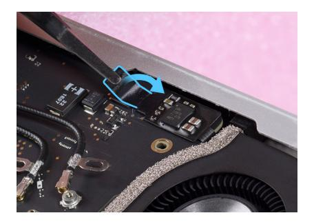
24. Gently slide the fan flex cable out of the connector.
