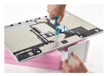
13. Place the computer upright. Hold the top and bottom edges of the housing. Then gently push the housing back and forth to ensure that it tilts back and forth smoothly.
