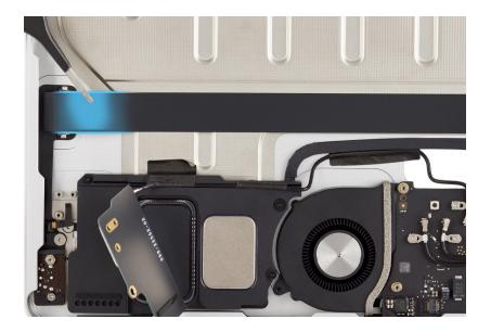
9. Slide the end of the power button cable into the connector on the audio board. Then flip down the locking lever.
