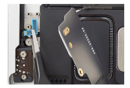
6. Use the T3 screwdriver to remove the upper T3 screw (923-05670) and the lower T3 screw (923-05669) from the audio board.
