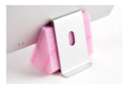
2. Lay the triangle support wedges used for display removal on their sides. Then place the housing on top of them as shown with the back of the housing facing down and the stand positioned between the triangle support wedges.
