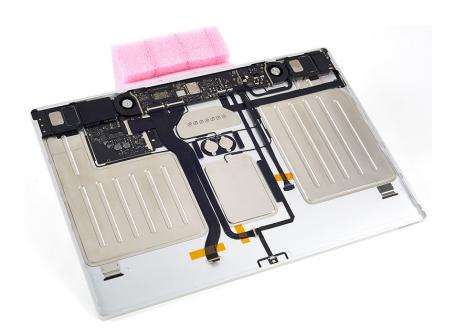
4. Use ESD-safe tweezers to peel off the polyester film tape on the fan flex cable.
