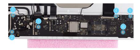
3. Use the 2.5 mm hex nut driver to partially reinstall four 2.5 mm hex nut screws (923-05556) (1-4) into the logic board.
