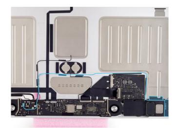
1. Use the T3 screwdriver to remove the three T3 screws (923-05574) from the Wi-Fi antenna.
