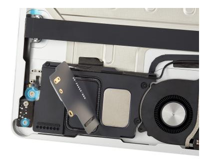
3. Use the 3.5 mm hex nut driver to partially reinstall the 3.5 mm hex screw (923-05671).
