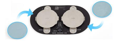
2. If you're reinstalling the same battery board, apply a new adhesive strip to the back of the battery board as shown. Fold down the adhesive tab (1) between the batteries.
