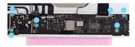
19. Use the 2.5 mm hex nut driver to remove four 2.5 mm hex nut screws (923-05556) from the logic board in the order shown.
