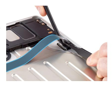
4. Remove the adhesive backing from the audio board flex cable. Then press along the length of the audio board flex cable to adhere it to the housing.
