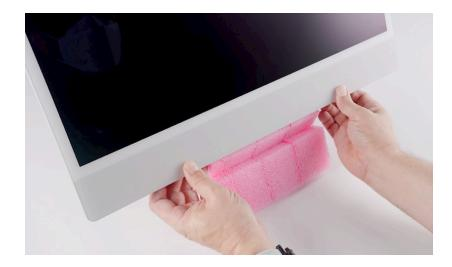
25. Ensure that the four edges of the display and housing are aligned. If they aren't aligned, repeat the removal and reassembly steps.
