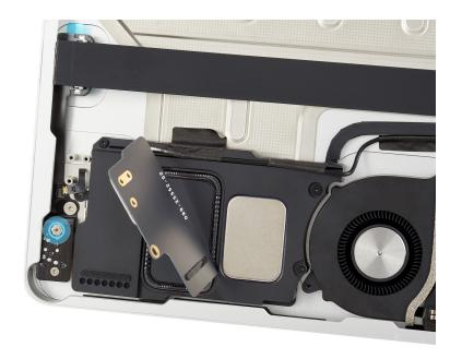
4. Plug the EarPods into the 3.5 mm headphone jack to ensure audio board alignment. Adjust the alignment of the audio board until the plug is easy to insert and remove.
