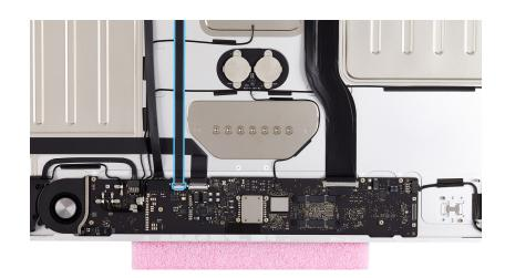
14. Slide the end of the audio board flex cable into the connector.
