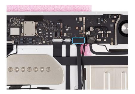
3. Squeeze both sides of the end of the display backlight flex cable and pull it straight out of the connector.
