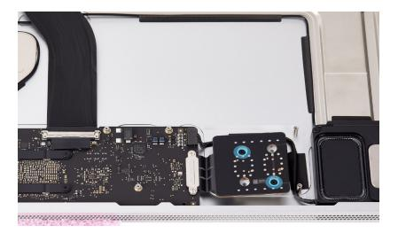
5. Reinstall the polyester film tape over the USB-C board.
