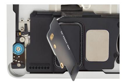
8. Insert the flat end of the black stick under the audio board to loosen the adhesive in the areas shown (1, 2). Then use ESD-safe tweezers to gently peel up the audio board and remove it from the housing.
