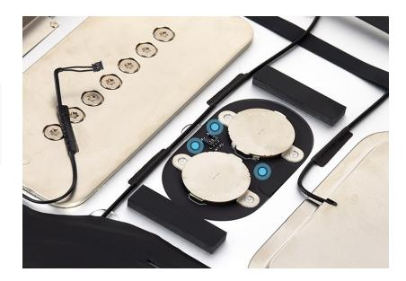
6. Press the end of the battery cable to the connector.
