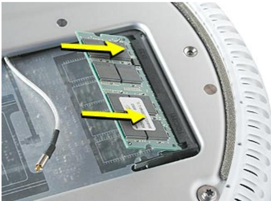
2. Press down gently on the memory until you hear it click into place under the two locking tabs on the sides of the slot (Figure 5).
