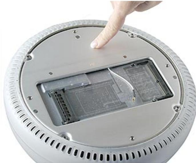
5. **Warning: Do not touch the screws on the bottom housing (Figure 4). Loosening these screws could cause the computer to overheat and damage internal components. Figure 4**
