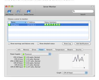
Server Monitor is installed in /Applications/Server/ when you install your server or set up an administrator computer. To open Server Monitor, click the Server Monitor icon in the Dock or double-click the Server Monitor icon in /Applications/Server/. From within Server Admin, choose View > Server Monitor.
