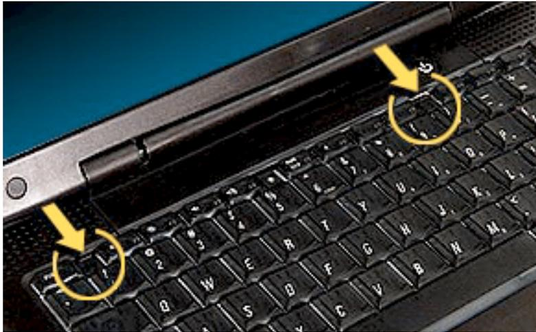
5. Lift the top portion of the PowerBook keyboard up slightly near the top row of keys and pull it back far enough to release the small tabs that hold the bottom of the keyboard in place.
