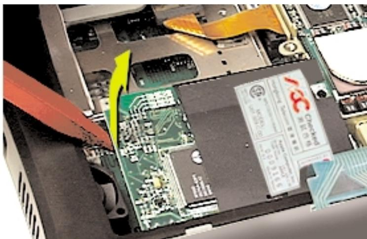
12. Grasp the keyboard connector handle and pull up to disconnect the keyboard from the logic board.
