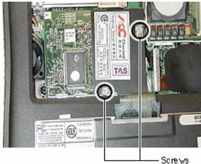
11. Use a flat-blade nylon tool to lift up the top left side of the modem and put the modem aside.
