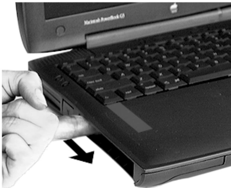
5. Lift the bottom portion of the keyboard up slightly and pull it back to disengage the five metal tabs holding the keyboard in place.
