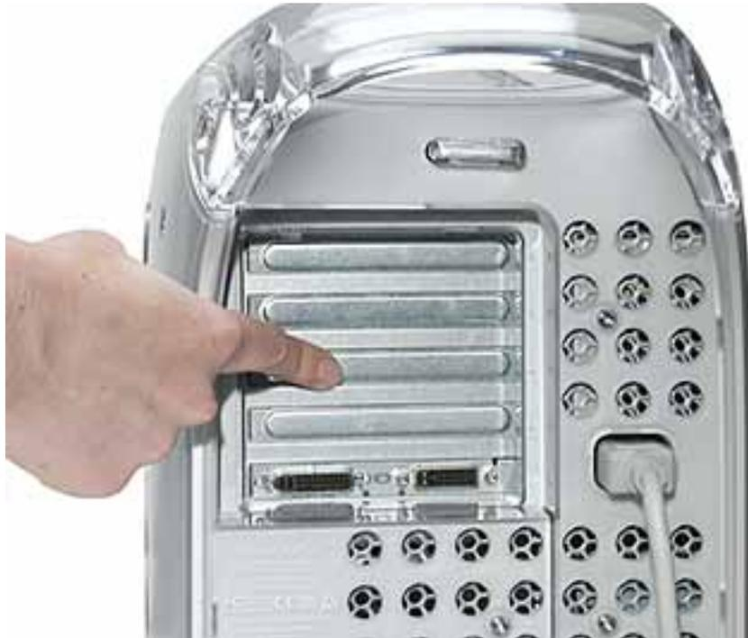
**Important:** To avoid electrostatic discharge, always ground yourself by touching the port access covers before you touch any parts or install any components inside the computer. To avoid static electricity building back up in your body, do not walk around the room until you have completed the installation and closed the computer.
