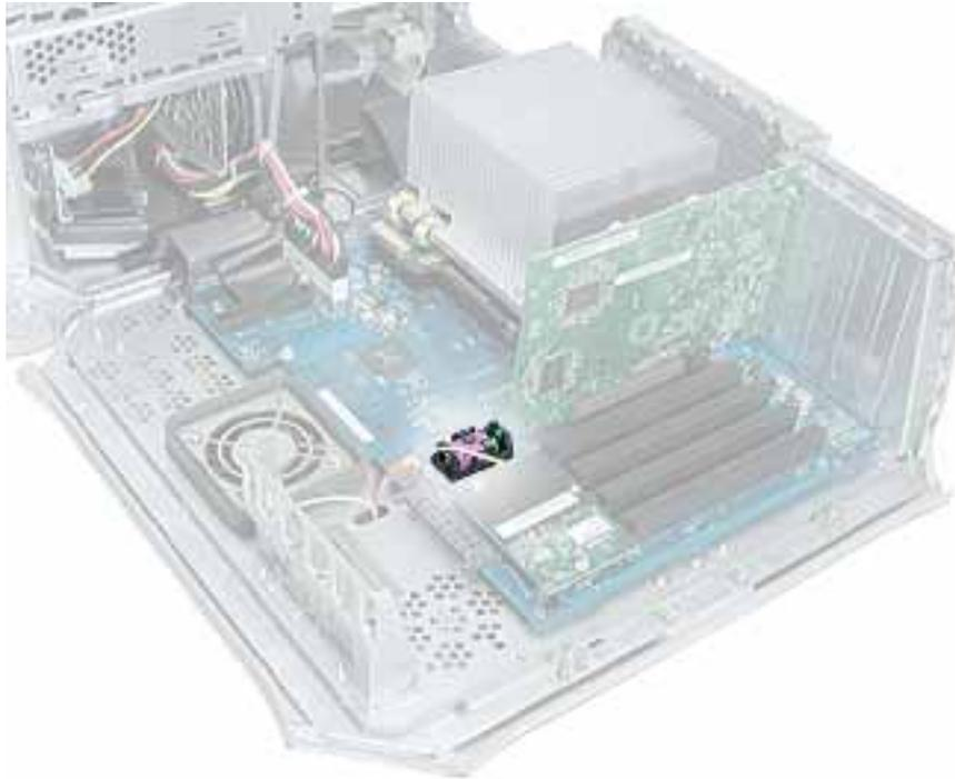
2. If a full-length video card extends over the battery, remove the video card as follows.
