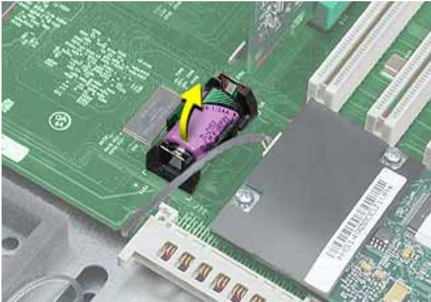
5. Insert the new battery into the holder, making sure the battery's positive and negative signs align with those on the holder.
