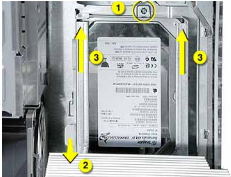
3. Rotate the carrier back from the chassis far enough to reach the drive cables.
