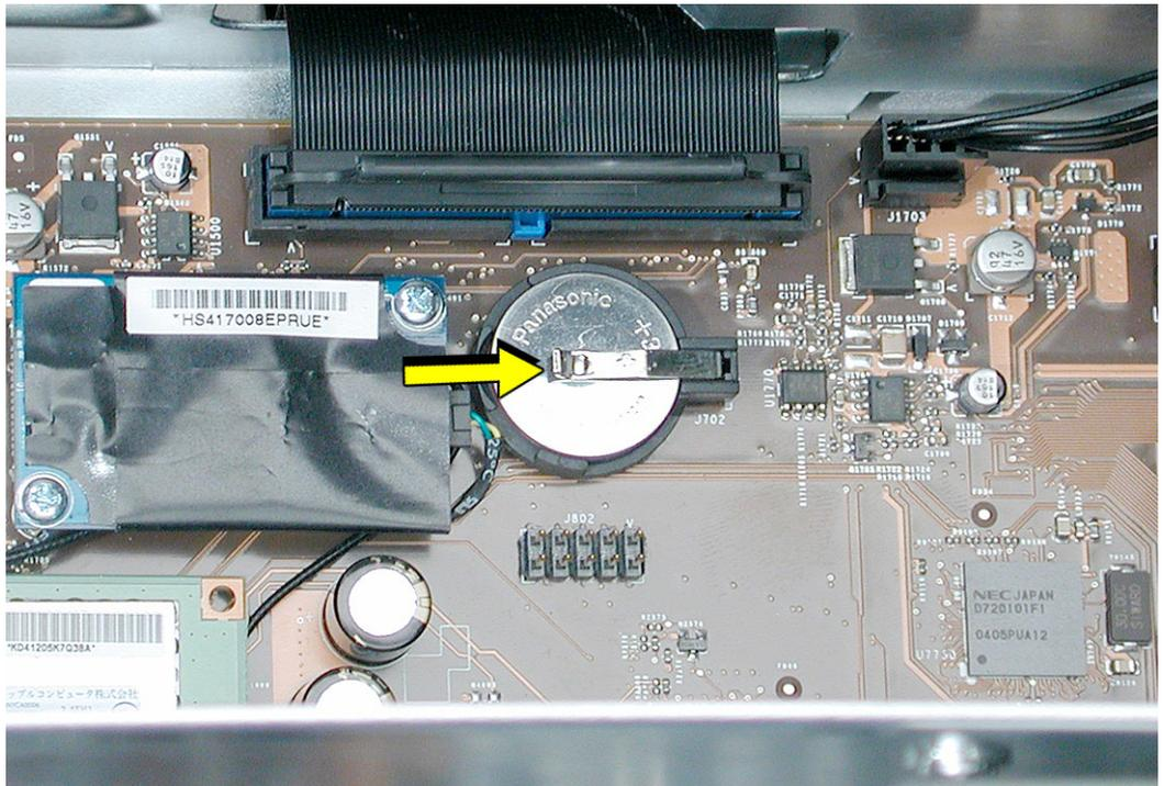
**Warning:** Installing the battery incorrectly may cause an explosion. Be sure the battery's positive and negative poles are correctly oriented in the holder. Use only the same type of battery or an equivalent recommended by the manufacturer of the original.
