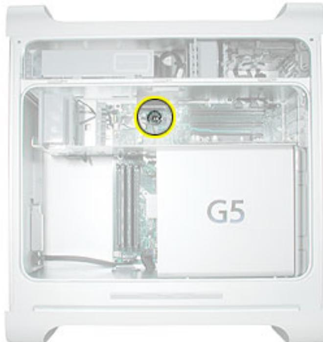
2. Insert a fingernail or jeweler's flat-blade screwdriver into the cut-out in the side of the battery holder and lift the battery slightly. **(Figure 5)**
