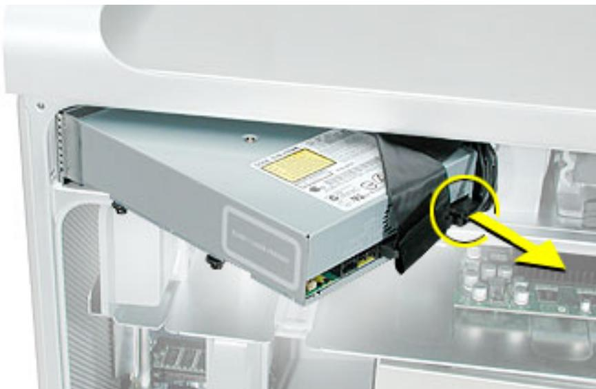
5. Route the drive ribbon cable out through the opening in the media shelf and remove the drive and ribbon cable from the computer.
