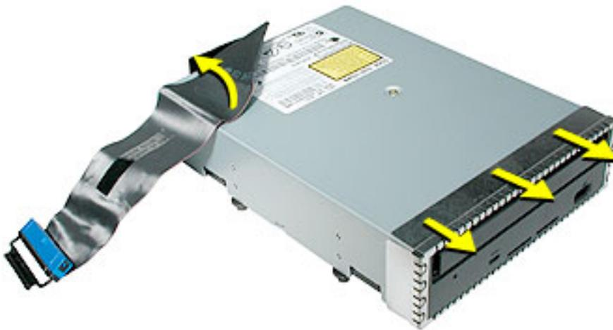
4. Insert the replacement drive part way into the optical drive bay. Bend down the free end of the ribbon cable, route it through the opening at the back of the media shelf, and connect the cable to the logic board.
