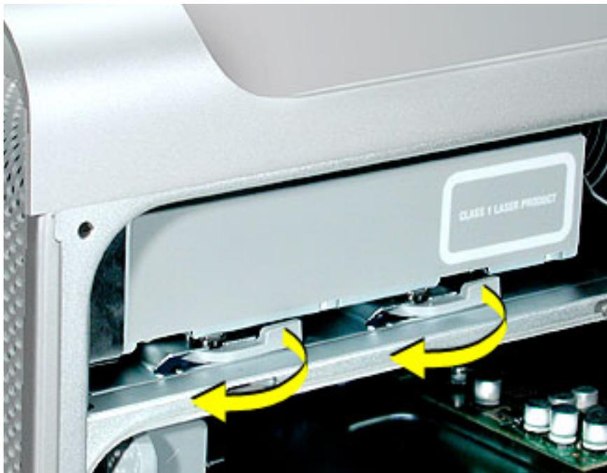
3. Place the fingers on one hand inside the opening for the optical drive cable and push the edge of the drive forward. The drive will move part way out of the media shelf. (Figure 6)
