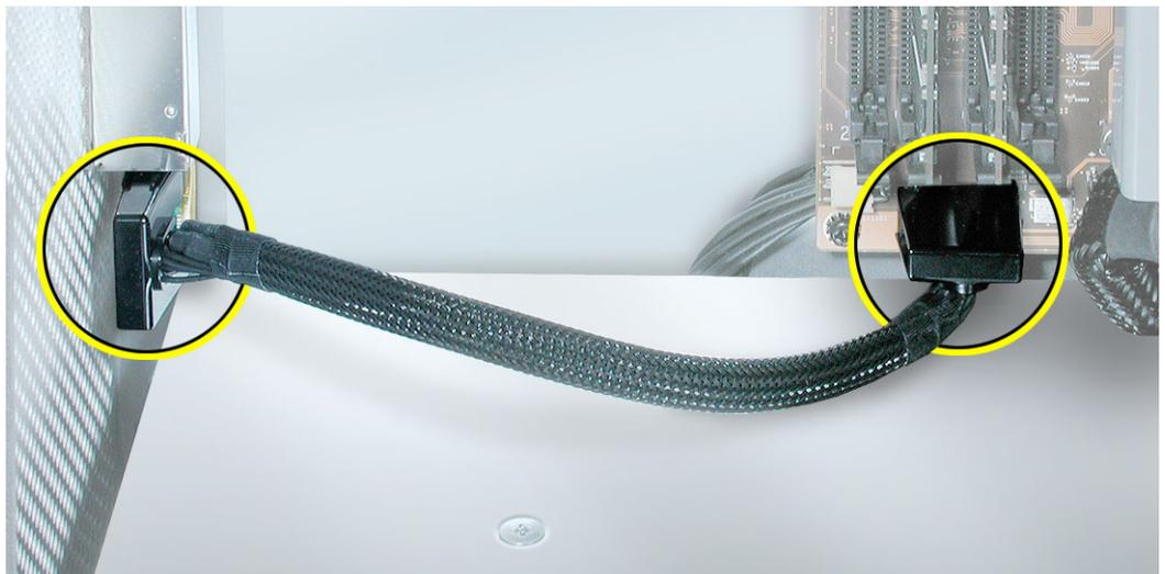
4. Disconnect the cable from the logic board. **(Figure 6)**
