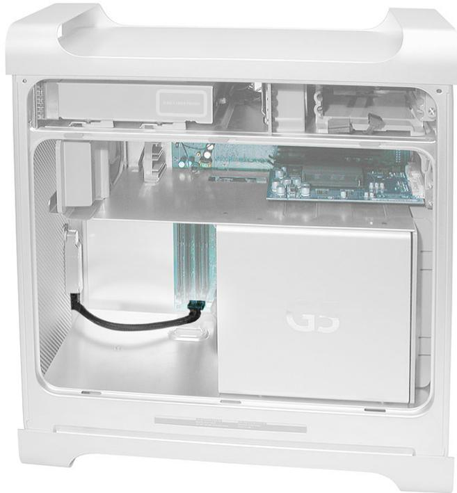
2. Carefully lay the computer on its side so that the open side faces up.
