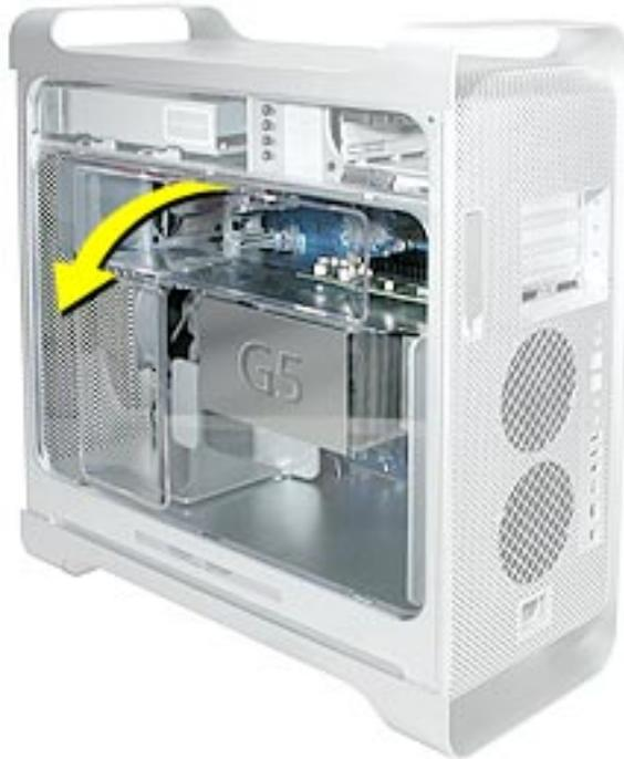
2. Install the replacement air deflector by inserting the three tabs on the bottom edge of the deflector into the three slots in the bottom frame of the enclosure. Then swing the deflector up flush against the top frame.
