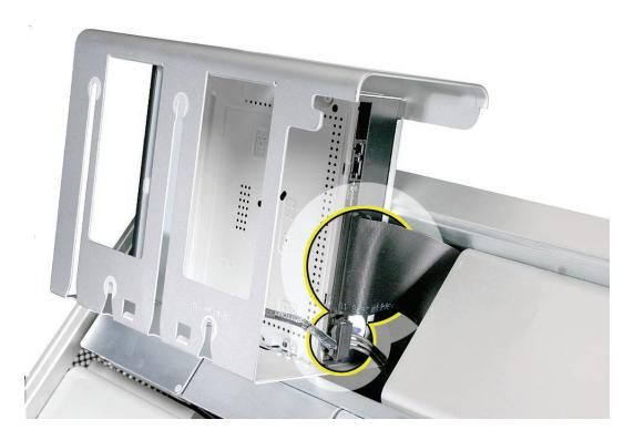
Slide the optical drive carrier over the guides and into place in the optical drive bay.
