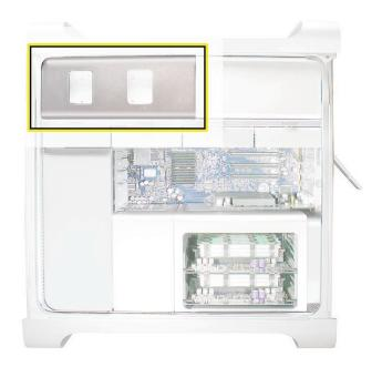
3. Pull the optical drive carrier part way out of the computer.
