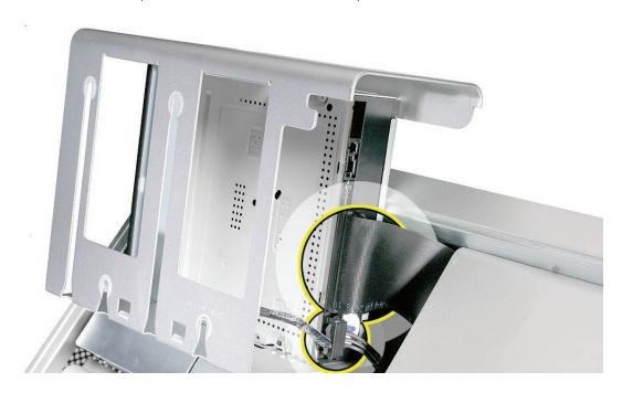
5. Remove the four mounting screws and remove the optical drive from the carrier.
