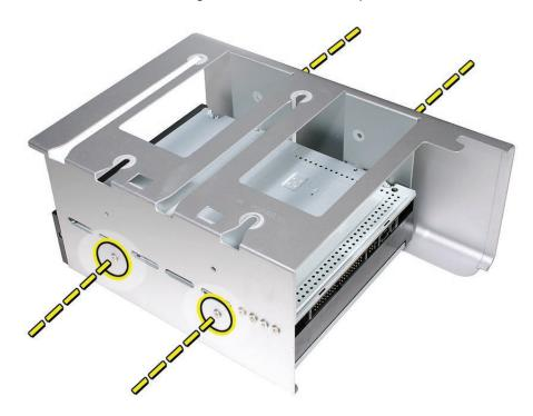
**Note:** If you are adding a second drive to the carrier, use the four screws stored on the back of the drive carrier to secure the drive to the carrier.
