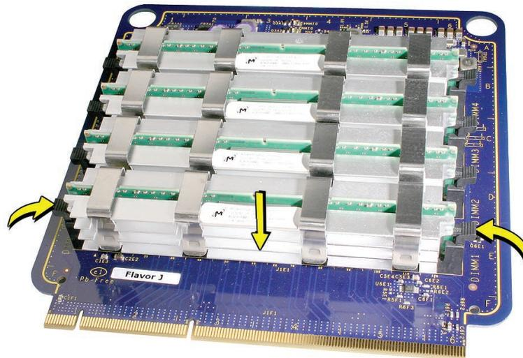
2. Insert the replacement riser card into position in the memory cage, pushing slightly until the card is seated in its logic board memory slot.
