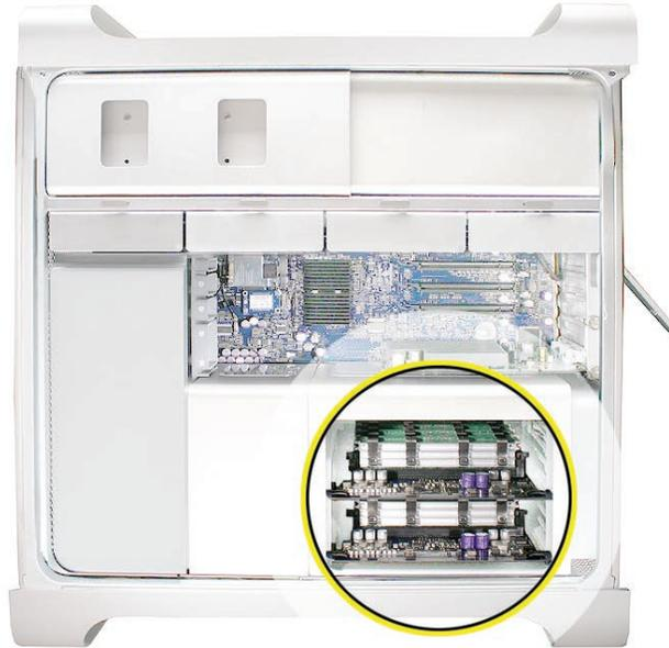
3. Holding the memory riser card by the two finger holes, pull it out of the memory cage and place the card DIMM-side-up on a soft, clean cloth.
